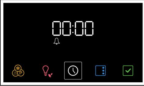
2. Turn the temperature knob to set the duration of the minute minder timer (from 1 minute to 23 hours).
