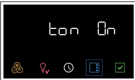
2. Turn the temperature knob to disable the sound associated with the touching of the symbols on the display.
