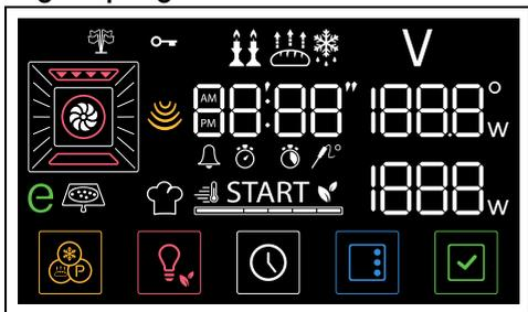
The parameters and values for the currently selected function will be indicated on the display. To use it, simply turn the functions and temperature knobs and/or press the buttons on the lower part of the display, depending on the operations to be performed by the appliance.
