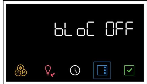
2. Turn the temperature knob to activate the controls lock function.
