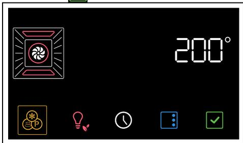
3. Turn the temperature knob to select the required temperature (from 50°C to 250°C).
