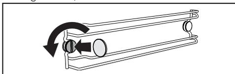
2. Carefully pull the frame towards the inside of the oven cavity to unhook it from front housing A.
