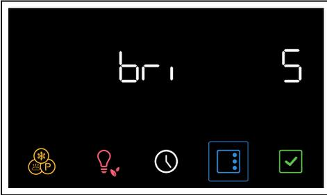
2. Turn the temperature knob to the right or left to select the desired brightness, from value 1 (low brightness) to value 5 (high brightness).
