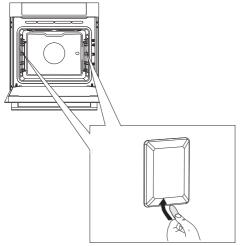
Use a flat screwdriver to release the bulb cover and remove it.
