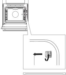
Remove the metal cap (the socket is in the front upper corner of the oven right wall).
